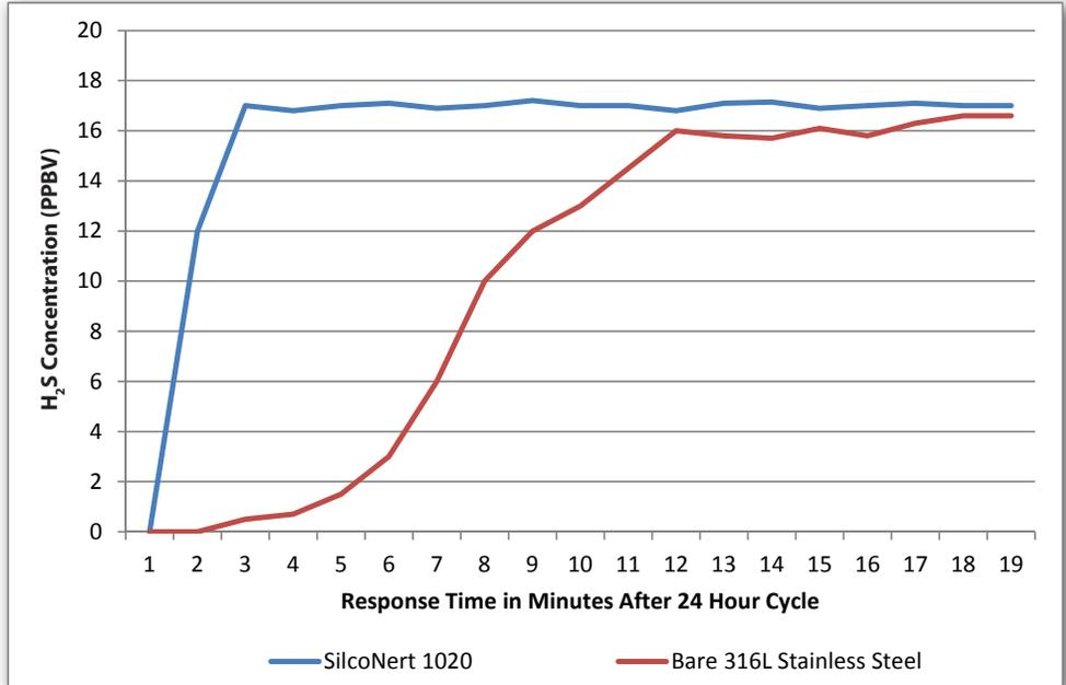
Figure 1 compares the response time of a calibration gas containing 17 ppbv of hydrogen sulfide delivered through a 316L stainless steel regulator and a CONCOA SilcoNert 1020 regulator after 24 hours. In this typical scenario, calibration was more than 10 minutes faster with SilcoNert 1020 than with 316L stainless steel.
