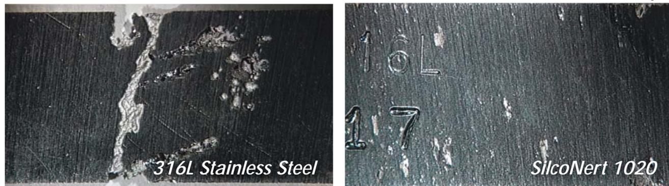
Figure 4 above shows the difference between an untreated 316L stainless steel test sample and a SilcoNert 1020 test sample exposed to an acid chloride solution per ASTM G 61.
