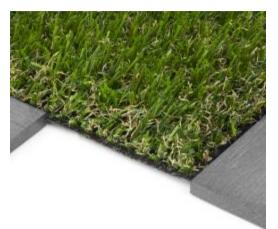
PermaLawn artificial grass consists of highquality synthetic filaments threaded into a backing layer which allows water to drain through. This backing layer is installed on a drainage layer which is usually comprised of compacted gravel. The artificial grass is then fastened down at any seams and along its perimeter.
