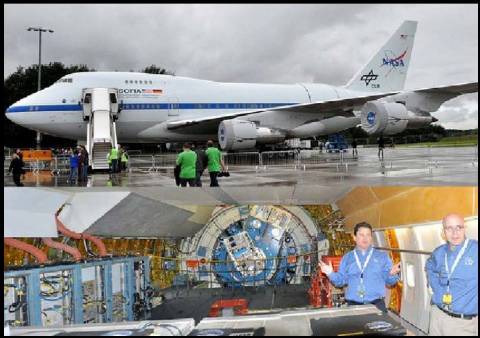
The SOFIA (Stratospheric Observatory for Infrared Astronomy) aircraft both inside and out. SOFIA carries a 2.5m IR Telescope. Photo: John Richards
