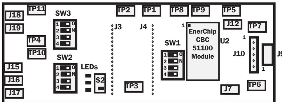
Figure 3: EnerChip EVAL-09 Connections, Test Points and Switches
