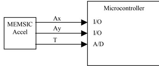
Figure 4: Zero g Offset Temperature Compensation Circuit
