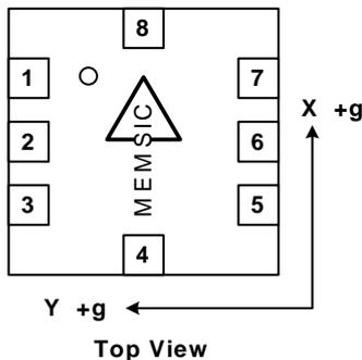
**Note:** The MEMSIC logo's arrow indicates the +X sensing direction of the device. The +Y sensing direction is rotated 90° away from the +X direction. Small circle indicates pin one (1).
