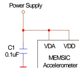
Figure 7: Power Supply Noise Rejection
