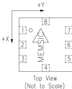
**Note:** The MEMSIC logo's arrow indicates the -X sensing direction of the device. The +Y sensing direction is rotated 90° away from the +X direction following the right-hand rule. Small circle indicates pin one (1).
