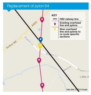
We'll build a new pylon near Drayton Lane, Drayton Bassett, install electricity cable onto it and connect each end to the existing network. The blue marker denotes the location of the pylon being replaced.
