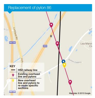
We'll build a new pylon near Dunton Coppice, off Kingsbury Road, install electricity cable onto it and connect each end to the existing network. The blue marker denotes the location of the pylon being replaced.
