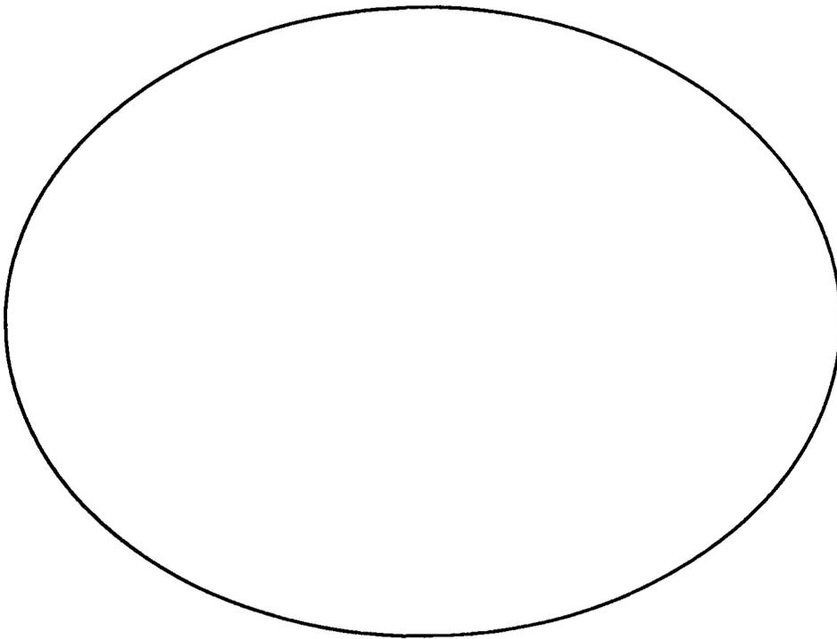
A precise mathematical construction of this curve is difficult. One fairly practical method is to employ the ellipse's 'focal property': a line from one focus to the perimeter and back to the other focus has constant length:
