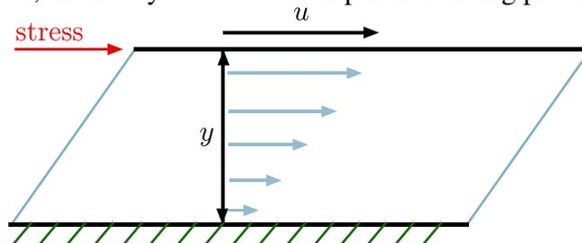
Dividing the speed of the top plate by the gap between the plates gives us the *shear rate*,  $\dot{\gamma}$ . We can measure the force (per unit area) required to make the top plate move along; the *shear stress*,  $\sigma$ .
