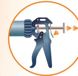
A Press lever clasp release and pull pressure piston out to maximum position.
