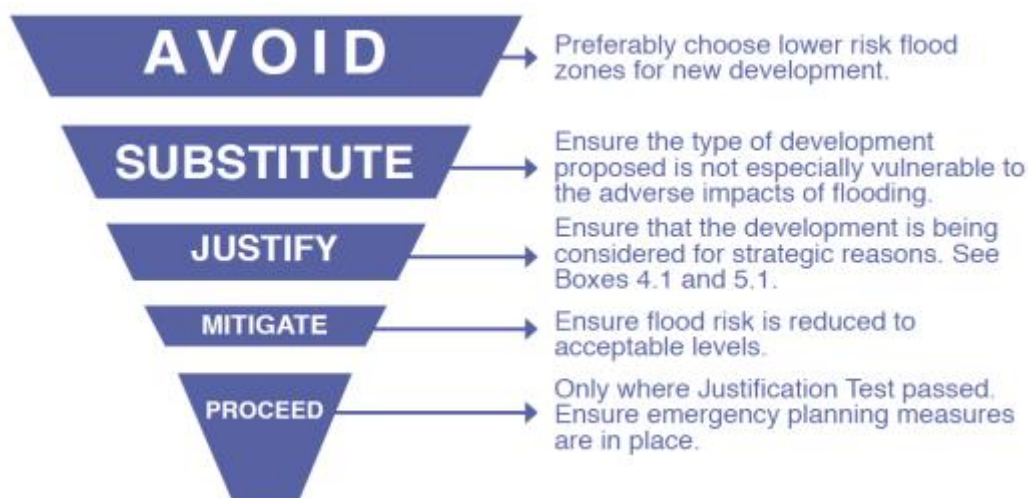
Figure 5-1 Sequential approach principles in flood risk management
