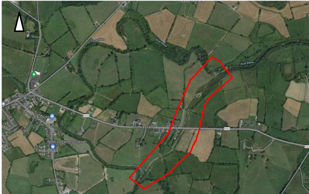
Figure 3-4 River Bilboa flood relief channel (Google Earth, 2022).
