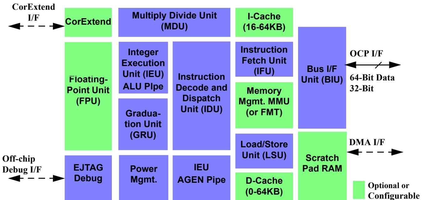
FIGURE 1. MIPS32® 74K® Processor Core Block Diagram
