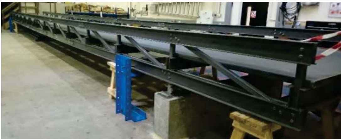
Figure 1: FRP Laboratory Footbridge.
