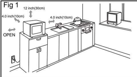
A 10-cm spacing should be kept between the appliance and right and back walls, and a 30-cm spacing kept on the top. Never dismantle the appliance's feet, nor block the air intake and exhaust opening. The left side must be open.
