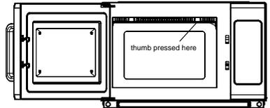
2. The left hand grasp the microwave, right thumb to press the arrow directions and forced to push back. And the left thumb hard pressed upward at the same time, put the right of oil blockage into the buckle of the front plate.
