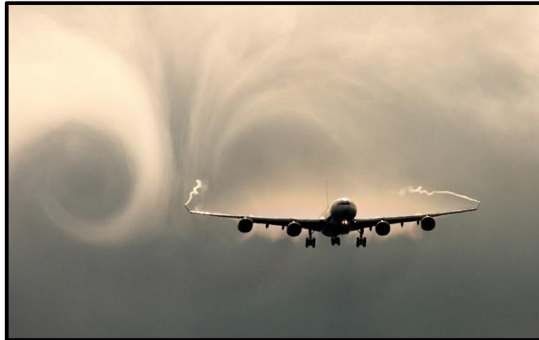
Figure 9: Wake vortices behind a landing aircraft
