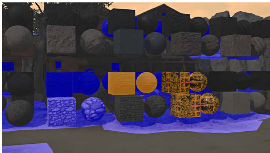
Figure 4 Overlay for validation of specular color. Blue means the value is below physically plausible range, orange indicates it is too high.
