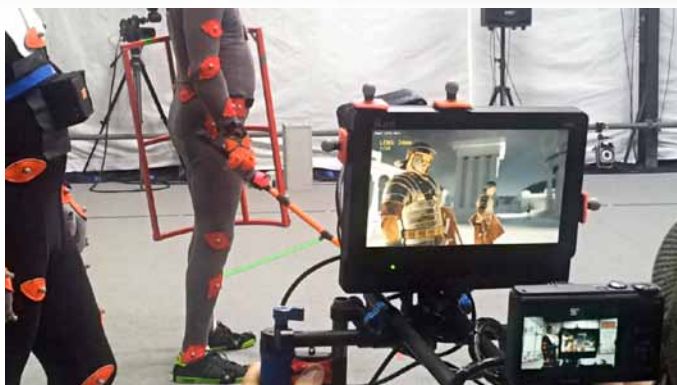
Crytek fabricated virtual camera hardware that allowed the director to »film« in the game engine.
