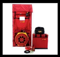
Model EU6112F with large cloth panel will fit larger doorways. The powerful 1240 W fan will test PRVs at higher pressure. It includes the new DM32 WiFi gauge. This 1240 W system is Ideal for larger enclosures up to 1450 m³ for inerts and 3000 m³ for halocarbons.
