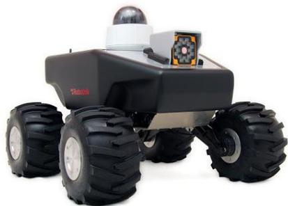
Figure 5 VINBOT, an autonomous yield estimation and NDVI mapping vineyard robot (VINBOT,2020)
