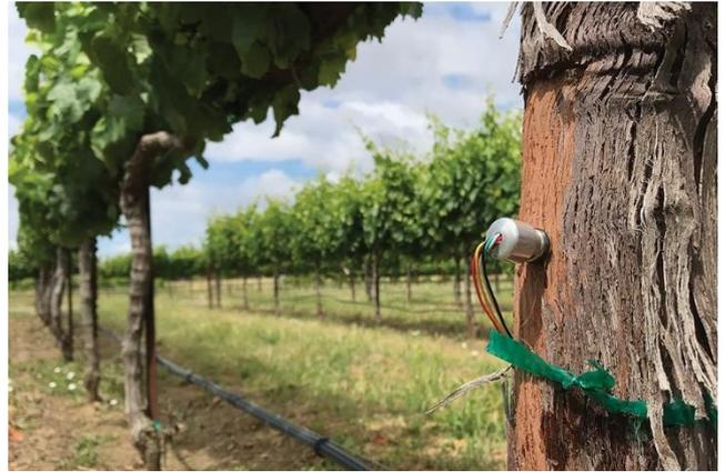
Figure 4 FloraPulse installed on a grapevine trunk, showing the sensor casing and wires (Picture by Michael Santiago in Growing Produce, 2019)
