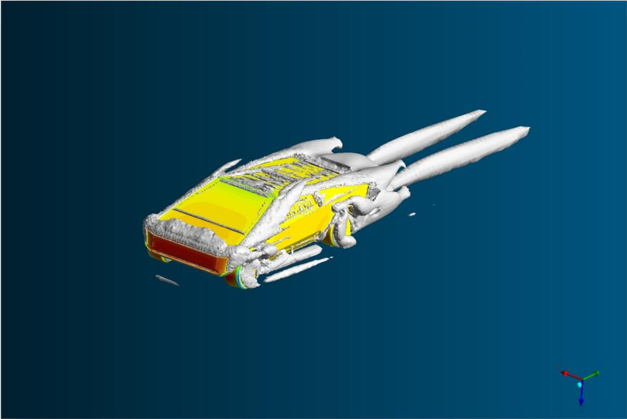
The wheels are simplified for CFD analysis and are not realistically represented. They will most probably have an impact on the vortex generation and aerodynamics.
