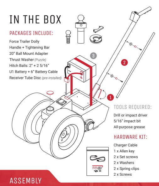
Slide the **handle** into the handle receiver tube and secure it with the provided **set screws** and **Allen key**. Plug the **handle cable** into the 3-prong port next to the dolly's volt meter. Use the remaining **washers** and **screws** to mount the **spring clips** to the handle for easy access to the **Tightening Bar**.
