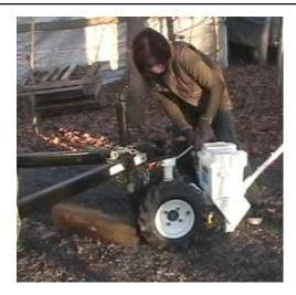
6. Tighten the ball mount as tight as you can. Test the stability by pulling up and down on the Parkit360 Force handle
