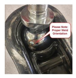
6. With your trailer jack, lower the trailer down onto the ball and lock it as you normally would. Again, please check that the weld spots on the ball are positioned correctly (as shown in step 5).
