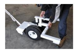
3. Use the forward hole to mount the ball. This is the most stable configuration. However, the rear hole may be used if the forward one is not practical to use due to space considerations.
