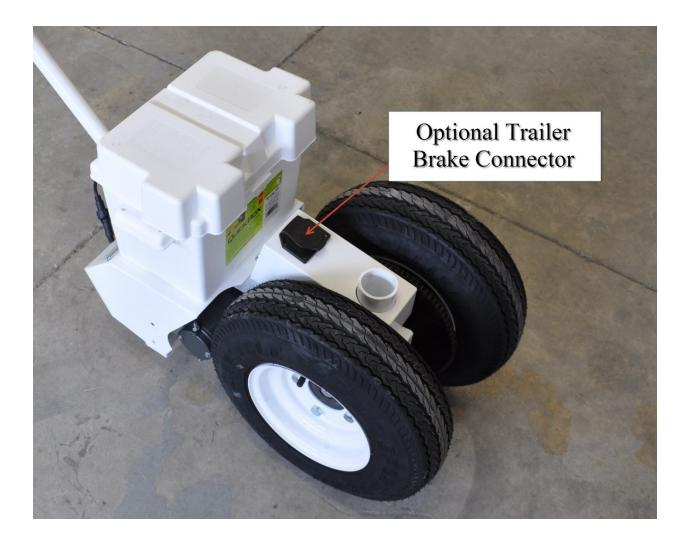
The Parkit360 Force features a connection for your trailer brake system. When connected and powered on, the trailer brakes will be engaged automatically whenever the unit isn't moving. When the motor is activated, in either direction, the brakes are released automatically.
