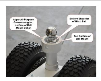
4. Please note that there are weld spots on the ball mount. These must be oriented properly before hooking up the trailer.
