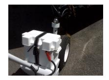
7. With pressure off the dolly (using the trailer jack), tighten the ball mount collar (counter-clockwise) using the supplied tightening bar. As you tighten it, you will see the gap between the top of the Ball Mount and the trailer tongue will close up.
