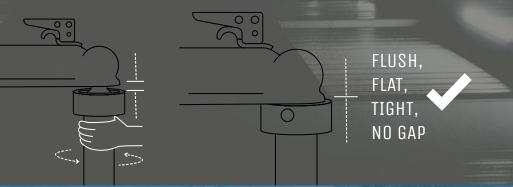
Have a **Step Down Hitch** or another obstruction preventing a flat connection? SEE THRUST WASHER INSTALLATION.
