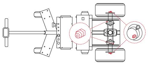
**Charging the On-Board Batteries:** Pull out on the **Battery Disconnect** to connect the batteries. Plug the **Charger Cable** into the Dolly and the opposite end into a nearby wall outlet. (*Page 7*)
