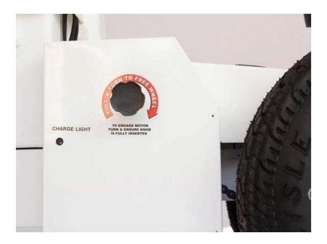
The knobs on the sides of the unit are used to change the wheels from engaged to freewheeling mode.
