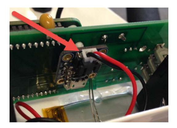
• Connect the battery charger port cable to the circuit board as shown below. Make sure the connector is oriented so that the Red wire is at the end labelled "+5" (RED) on the circuit board.
