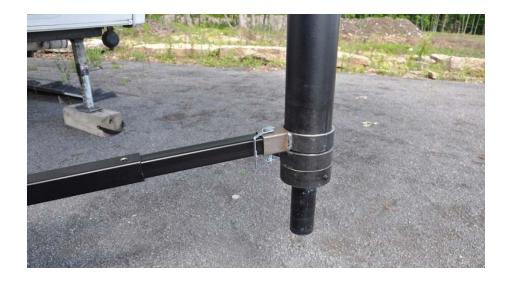
**Important:** Before attaching the stabilizer bars, please check to make sure they are oriented properly by checking the fit at the front landing legs. The tab at the leg end should fit to the outside of the front landing legs (see photo in step 3).
