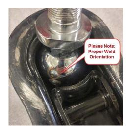
6. With your trailer jack, lower the trailer down onto the ball and lock it as you normally would. Again, please check that the weld spots on the ball are positioned correctly (as shown in step 5).
