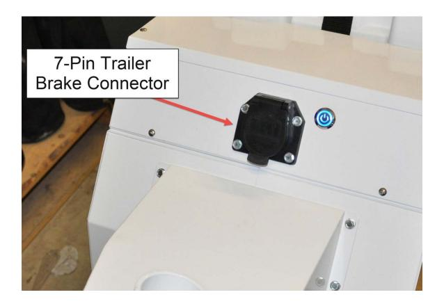
The Parkit360 Transformer features a connection for your trailer brake system. When connected and powered on, the trailer brakes will be engaged automatically whenever the unit isn't moving.
