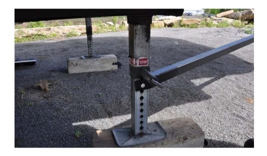
**Important:** As shown in the picture, make sure to install the stabilizer bar as close to the top of the leg as possible, ideally, right up against the hydraulic part of the leg. Once the stabilizer bar is secured at both ends, repeat steps 2 and 3 for the other stabilizer bar.
