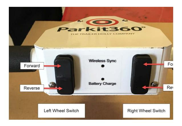
Pressing the top of one of the wheel switches will result in that wheel moving the unit forward, and pressing the bottom of one of the wheel switches will result in that wheel moving the unit in reverse.
