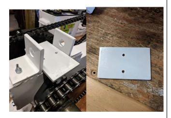
3.) Place receiver back inbetween the brackets on top of the plate. reinsert bolt through the adapter.
