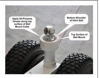
4. Please note that there are weld spots on the ball mount. These must be oriented properly before hooking up the trailer.
