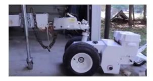
7. With pressure off the dolly (using the trailer jack), tighten the ball mount collar (counter-clockwise) using the supplied tightening bar. As you tighten it, you will see the gap between the top of the Ball Mount and the trailer tongue will close up.
