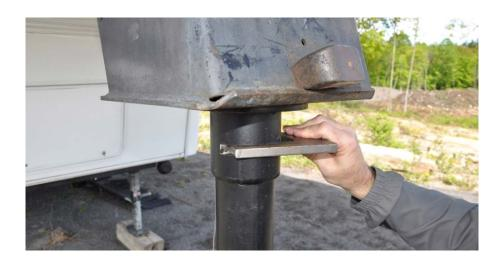
Attach and install the stabilizer bars. Begin by attaching the front end (the Kingpin end) of the stabilizer bar in the Kingpin Adapter Collar using the supplied D-Clips as shown below:
