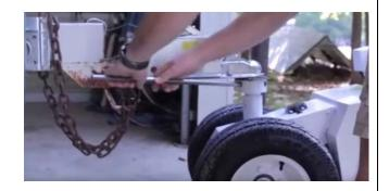
6. Tighten the ball mount as tight as you can. Test the stability by pulling up and down on the Parkit360 Force handle
