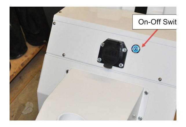
You will also hear a relay click inside the control module. This is the automatic brake system engaging. If your 7-Pin trailer plug is connected to the Transformer, the trailer brakes will be activated as soon as the power is turned on.
