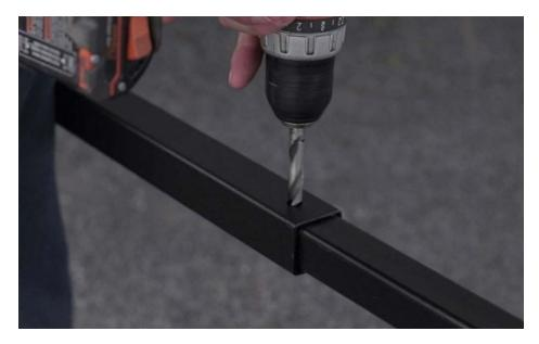
The hole must allow a 3/8" pin, so pick an appropriate drill bit (13/32") and using the top hole as a guide, drill through the inner stabilizer bar tube.
