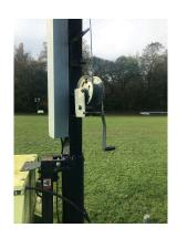
Step 4 Turn the winch handle anti clockwise to lower the mast until it is fully housed.
