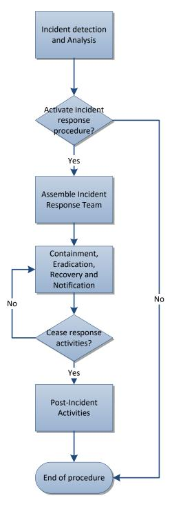
Figure 1 – Incident response flowchart
