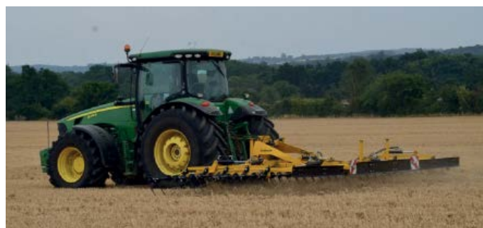
The new 9m mounted version of the Claydon Straw Harrow is seen here working in '80-acre', a field which has been managed using the Claydon Opti-Till® System for 20 years, after the previous crop of LG Skyscraper winter wheat had been harvested. Following 2.4mm of rain overnight the lack of dust was noticeable, even at 25km/h!
