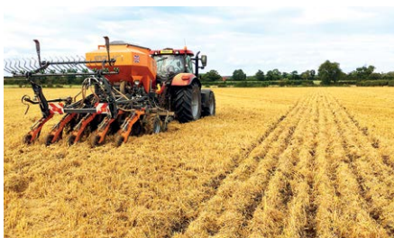
The Pro-Til with its wide row spacing and high clearance through the machine gives it the advantage in dense straw situations
