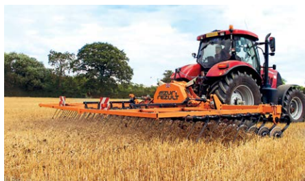
The Rezult rake is a useful tool for stubble management to spread uneven chopped straw and to encourage weeds to chit for a stale seedbed
