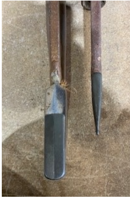
Comparison Photos of Weaving OEM Tine and the BTT Replaceable Tine and VOS 19mm tip after 800 acres. Also, a photo showing the wear between the VOS 19mm (after the 800 acres) trial tip and a new unused VOS 19mm tip.
