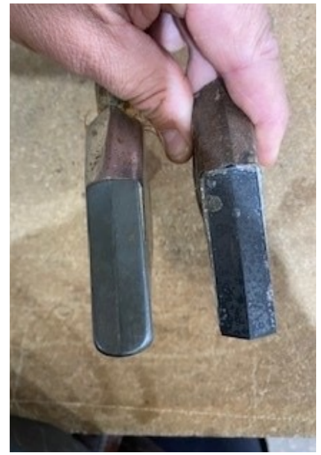
Comparison Photos of Weaving OEM Tine and the BTT Replaceable Tine and VOS 19mm tip after 800 acres. Also, a photo showing the wear between the VOS 19mm (after the 800 acres) trial tip and a new unused VOS 19mm tip.
