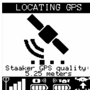
When a good GPS signal is found and the drone is ready for takeoff, the status LED will flash green. The following screen will appear on the tracker:
