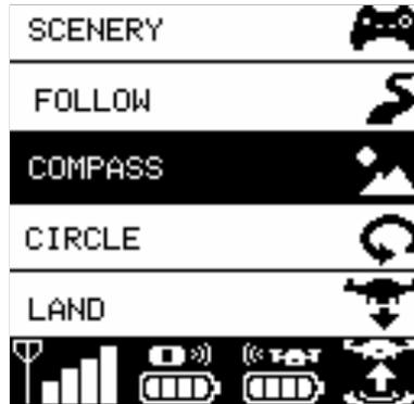
You can use **△** and **▽** buttons to move up and down in the mode selection menu. You can also press **M** to move down in the menu. To engage the selected option press **▶**. Once selected the drone will change mode and continue following you if it is unpaused.
