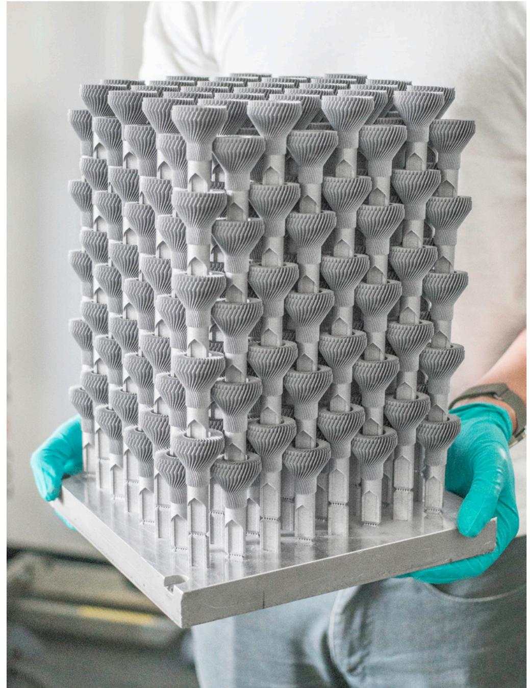
Production build of 384 Heatsinks. Manufactured by Progressive Technology on an EOS M280.
