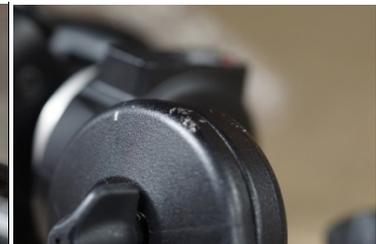
Indents in legs can influence use and should be noted by Hirecamera on the supplied Condition Report. Scratches with less than 2mm depth on tripod heads and legs are considered general wear and do not need to be specifically noted.
