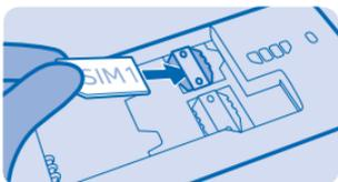
4. To insert a second SIM, slide the SIM in with the contact area face down.
