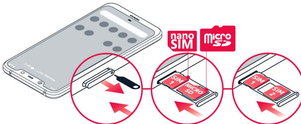
1. Open the SIM and memory card tray: push the tray opener pin in the tray hole and slide the tray out.
