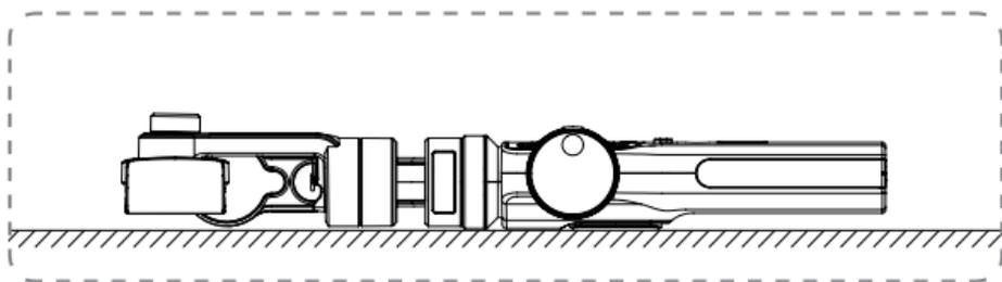
After activating stabilizer and entering stand-by mode, put the stabilizer on the ground and wait for 30 seconds, then the initialization of stabilizer is finished.
