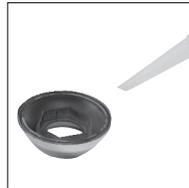
**6** Ensuring the fibre washers are positioned within the valve inlets, offer the valve into position. Tighten the fixing nuts using a suitable tool taking care not to overtighten.
