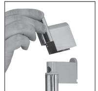
**8** If required, optional outlet flow regulators can be purchased from the Aqualisa customer helpline on 01959 560010. Fit the relevant flow regulator into the brass housing ensuring the O'ring faces the incoming flow. Connect the flow regulator assembly to the valve outlet ensuring the hose washer is correctly fitted.
