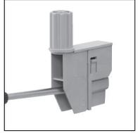
**3** Ensuring the lever is in the upright position, pass the rail through the handset holder.
