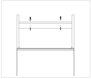
Secure the unit to the wall using the fixing kit provided. Screw through the back brace as shown in the diagram.
