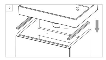
Apply the rubber extrusion to the side panels prior to applying silicone.
