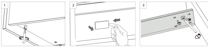
Ensure to release CAM bolt or L-bracket on bottom face of drawer first before releasing drawer fascia.
