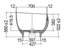
Dimensions: All dimensions in mm tolerance  $\pm 5\%$  for below 200mm and  $\pm 3\%$  for above 200mm. Note: Due to a continuing development programme to improve design and performance, the manufacturer reserves all rights to vary specifications without prior information.
