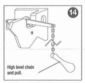
Secure the fulcrum bracket in place using the screw and flat nut provided, hook the fulcrum arm onto the C-link and clip the fulcrum arm into the fulcrum bracket, attach the high level chain and pull.
