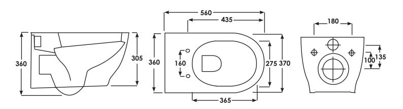
Dimensions: All measurements are in millimeters and are subject to normal manufacturing variations.
