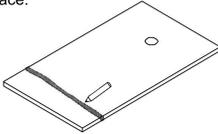
4) Check that your markings are correct and then mask off the cut line to protect the tray surface.
