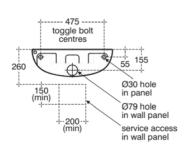
back view showing fixing in panels
