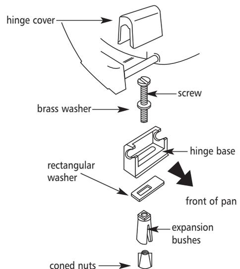
1. Locate top of expansion bushes into underside of hinge base and retain by inserting screws through washers, hinge bases and rectangular washers, then loosely tightening the coned nuts to engage the "wings" in the expansion bush slots.
