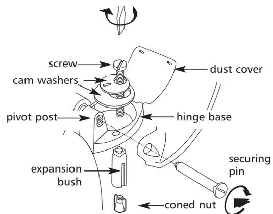
1. Position hinge base with pivot post between seat and cover pivot bases and align holes.
