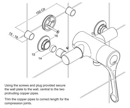
Run a bead of sealant onto the back of the concealing plates (16) close to the outer edge.
