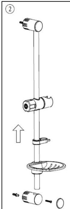
Place the slider bracket onto the rail, ensuring the wider opening of the handset holder is located upwards.
