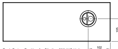
Push Button Position for Slimline 500 WC Unit if using Geberit Dual Flush Montage Cistern
