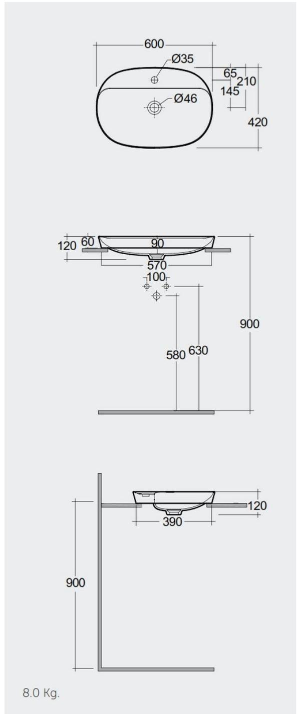
Dimensions: All dimensions in mm tolerance  $\pm 5\%$  for below 200mm and  $\pm 3\%$  for above 200mm.
