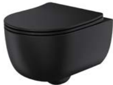
RIVIERA RIMLESS ROUND WALL HUNG PAN MATTE BLACK INCLUDING SOFT CLOSE SEAT 355w x 320h x 490d Bolt Centre 180mm Matching Basin - Page 47
