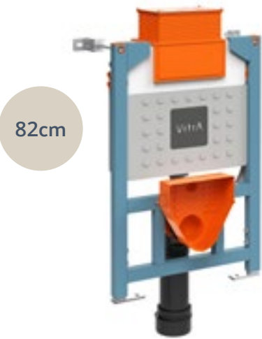
Reduced-height frame, floor & wall fixation, 82cm, 3/6 litre H: 820mm W: 500mm P: 160-190mm
