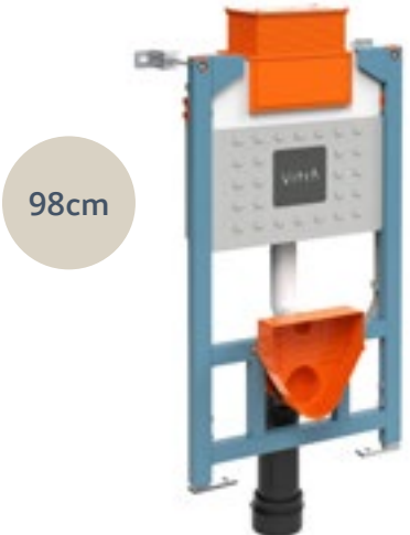
Reduced-height frame, floor & wall fixation, 98cm, 3/6 litre H: 980mm W: 500mm P: 160-190mm
