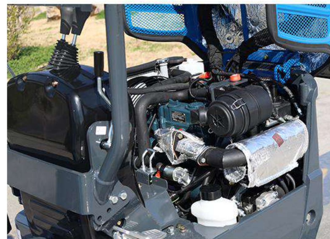
5 Fully openable bonnet The fully-opening bonnet opens wide to the rear, making it easy to carry out daily inspections and part replacements around the engine and fuel system.
