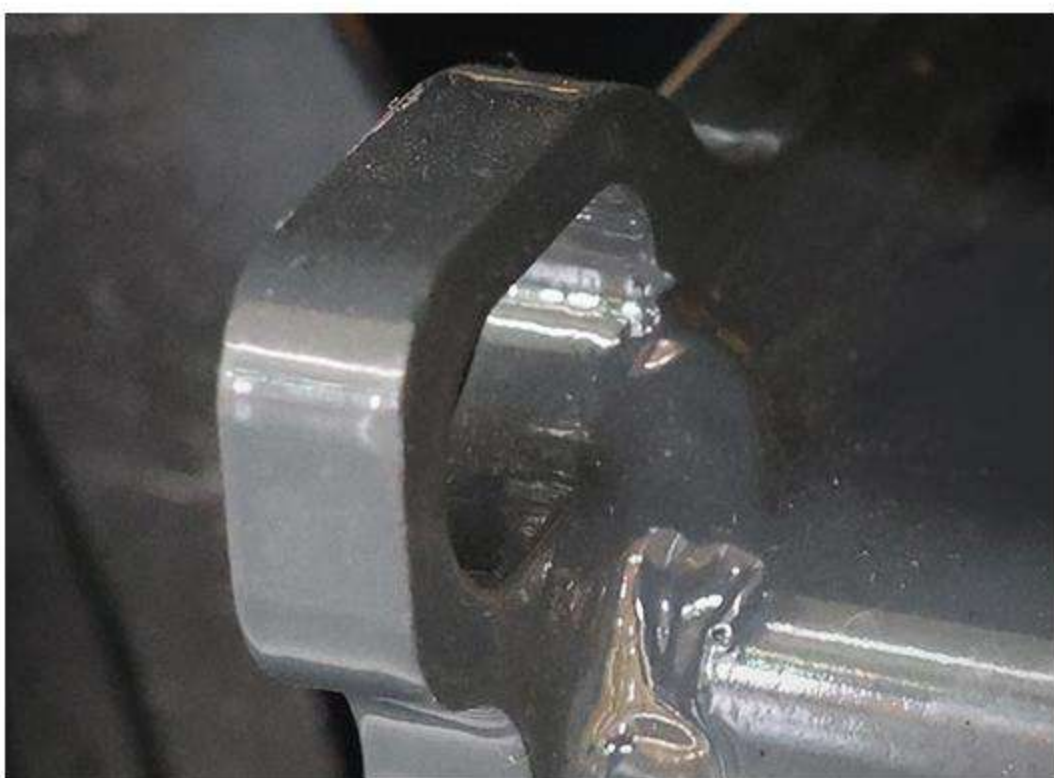
8 Added lower plate lifting port When the excavator needs to transport something stuck in mud, landslide or other emergency situations, the lifting port can be connected to a wire rope or hook to cooperate with the crane for safe lifting.
